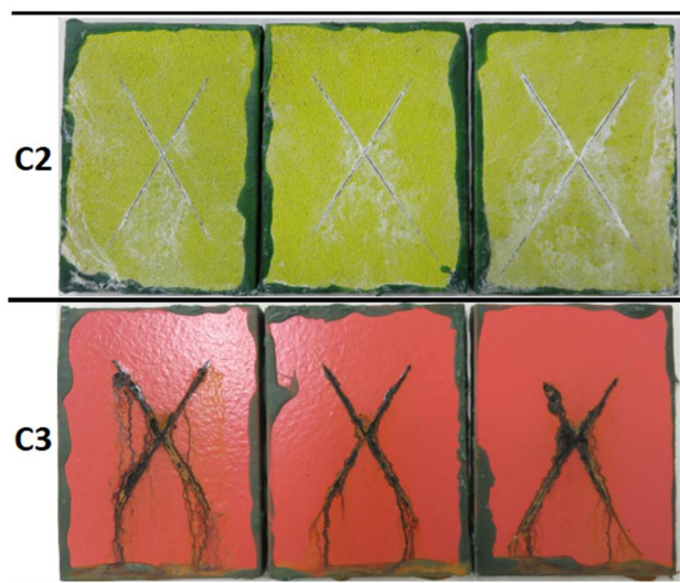
Figure 9. Visual appearance of the coatings surface without incision at different evaluations during 1440 h of exposure to salt spray, according to the ISO 9227 standard.
