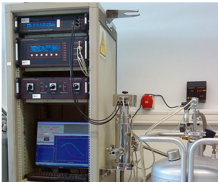
Figure 2.12. Setup of the Alpha-A Novocontrol dielectric analyzer used in this work.
