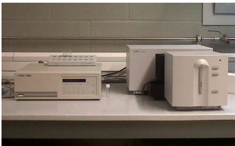
Figure 2.4. UV-Vis equipment used in this work.
