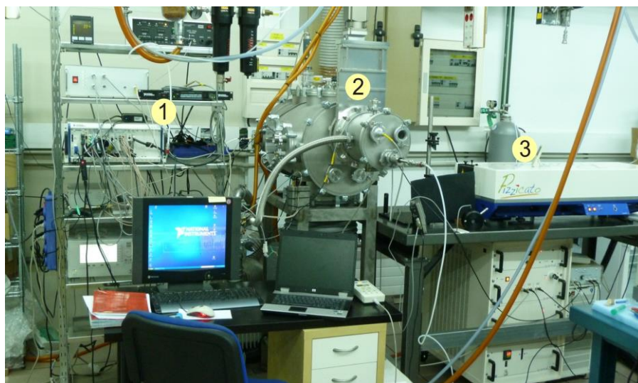
Figure III.4 Picture of the FTMW spectrometer at the University of the Basque Country (UPV/EHU), with numbering of the main components (1: Electronic tower with the electronic equipment, 2: Vacuum chamber, 3: Ultrafast laser vaporization set-up).
