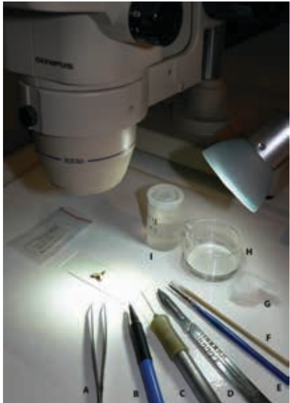
Figure 2.10 Selected instruments and basic material for fossil micropreparation. A, fine tip curved tweezers; B, 0.5 mm mechanical pencil with a steel needle; C, pin vise; D, scalpel with removable blades; E, fine paint brush with solvent-resistant hair; F, bamboo stick cotton bud; G, cotton pad; H, acetone; I, consolidant Paraloid B72 in acetone at 5–10% weight by volume (w/v) ratio.
