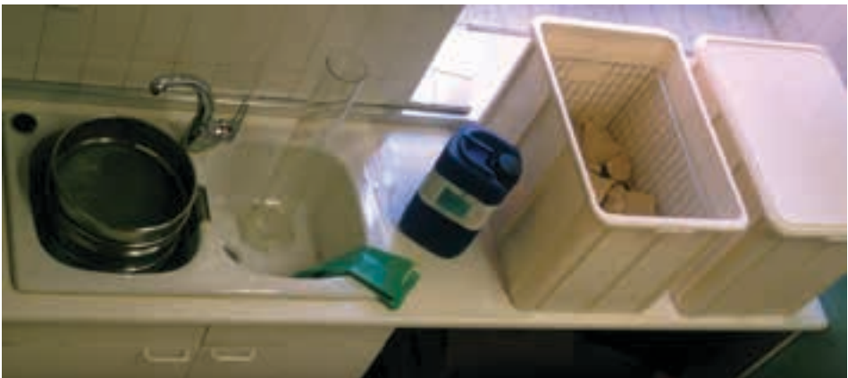
Figure 2.5 Wet laboratory space with a series of sieves, a graduated cylinder, and the reactive chemical (black plastic container) for extraction of microscopic fossil remains from the rock samples.
