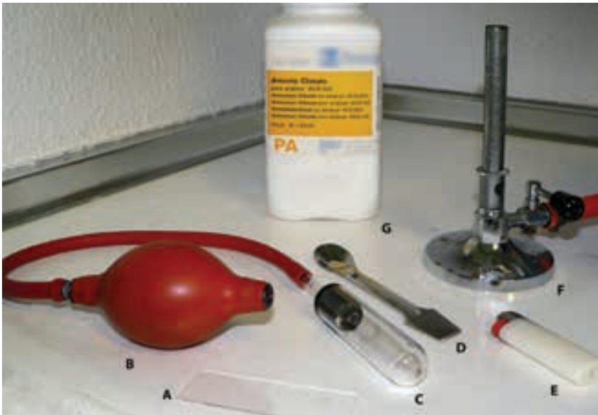
Figure 2.17 Basic equipment for whitening fossils prior to photography. A, microscope slide for mounting the specimens; B, rubber hand pump; C, customized test tube with a hole at the end for heating ammonium chloride; D, double-ended spatula and spoon; E, lighter; F, Bunsen burner; G, ammonium chloride reactive.
