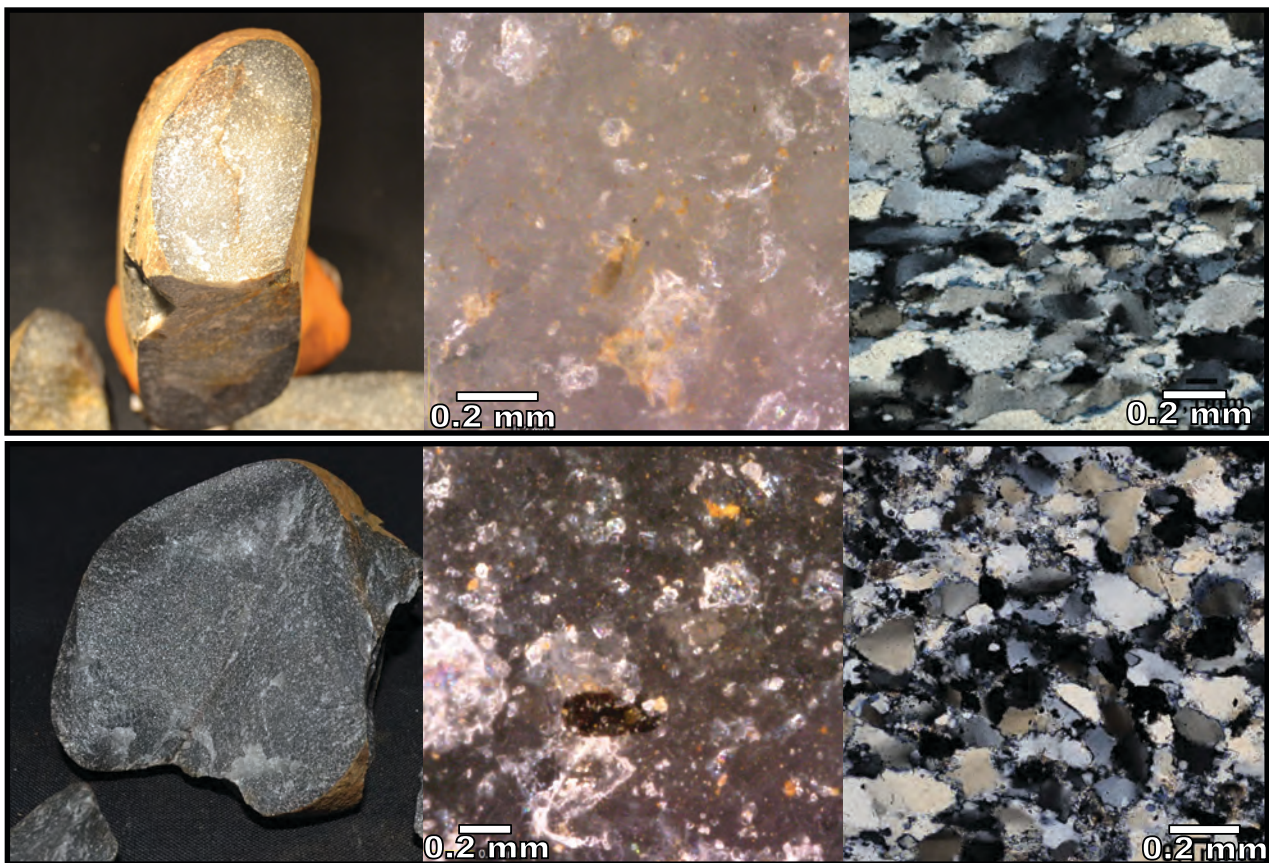
Figure-6.29: Pictures at different magnifications of the samples DC75_02 and DC75_05 from the Pontón conglomerate. The first sample is a BQ type (maybe RQ type) with fine quartz grain size heterogeneously distributed. The second sample is a BQ type with fine quartz grain sizes.
