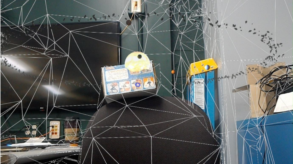
Figure 34: Spatial Mapping occlusion example at the SmartLab. We can see the sun being partially occluded by the box over the chair
