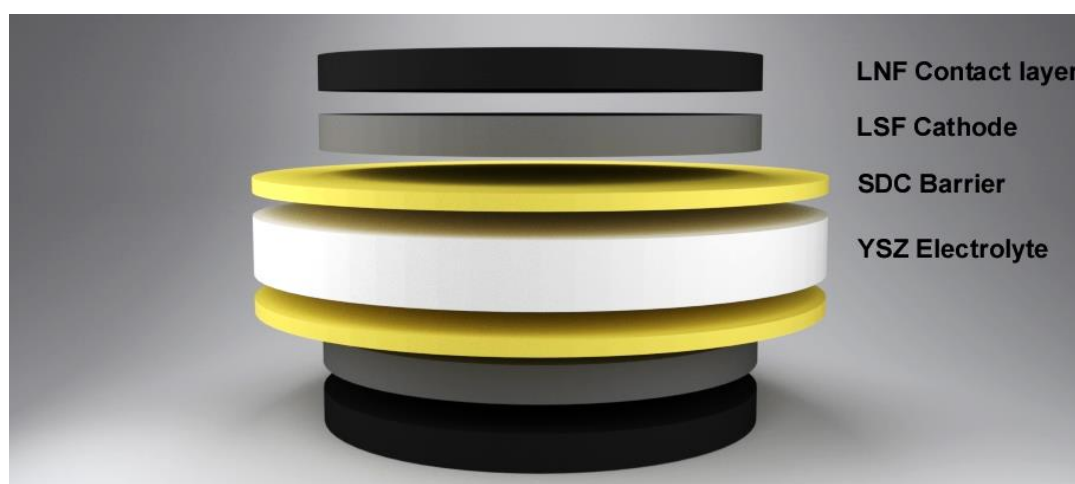
Figure 3.1.- Schematic for an electrolyte supported SOFC design.
