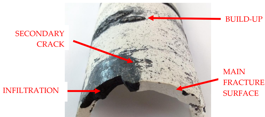
Figure 1. Picture of a cracked roller showing both aluminum build-up due to adhesion and aluminum infiltration across the full thickness of the roller wall.
