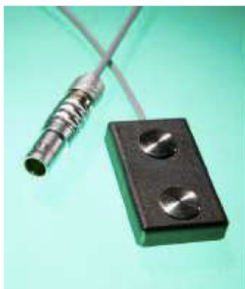
Figura. 2-13. Sensor EMG superficial. [http://www.brainclinics-products.com]
