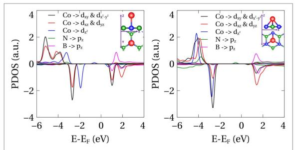
**Figure 5.** Projected density of states (PDOS) onto 3d orbitals of Co and  $p_z$  orbitals of first neighbour N and B atoms once for atop N (left) and once for hollow (right) adsorption sites, as obtained from the spin-polarized DFT calculations. Positive values correspond to majority-spin and negative values to minority-spin. The insets shows the adsorption site, where the red sphere represents the Co adatom, while the blue and green spheres represent N and B atoms, respectively.
