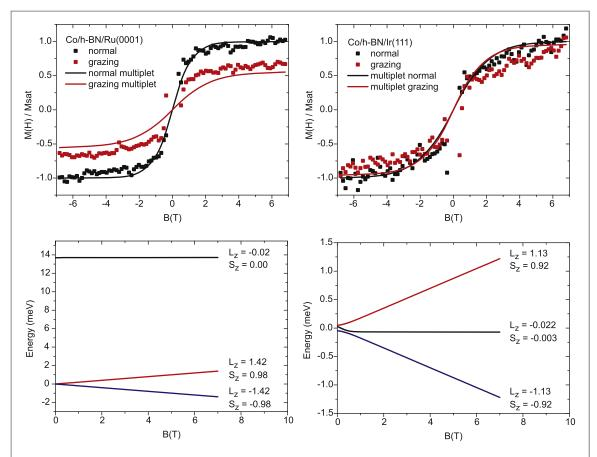
$\label{eq:figure 4.} \textbf{Figure 4.} \ Upper panels: magnetization curves, (dot) experimentally acquired and (line) obtained from multiplet calculations, for Co on h-BN/Ru(0001) and h-BN/Ir(111) at both normal and grazing incidence . Lower panels: corresponding field splitting of the Co lower states obtained from multiX multiplet calculations.$
