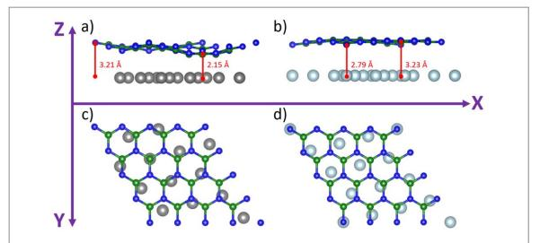
**Figure 1.** Side ((a) and (b)) and top ((c) and (d)) views of the  $4 \times 4$  supercell for h-BN on the Ru(0001) ((a) and (c)) and Ir(111) ((b) and (d)) surfaces, after relaxation of the h-BN monolayer in the Z direction. Green and blue spheres represent B and N atoms, respectively, while grey and light blue are the top most layer Ru(0001) and Ir(111) surface atoms. The side views, (a) and (b), clearly show the different corrugations of h-BN on Ru(0001) and Ir(111), respectively.
