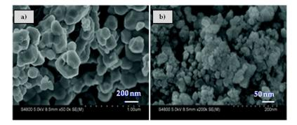
**Figure 5.** SEM images for LaCoO<sub>3</sub> perovskite prepared by (**a**) conventional method and (**b**) nanocasting, respectively. Adapted from [65]. Copyright (2013) Royal Society of Chemistry.
