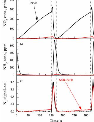
Figure 12. (a)  $NO_x$  (NO + NO<sub>2</sub>) and (b) NH<sub>3</sub> outlet concentrations, and (c) MS signal of N<sub>2</sub> for the single-NSR and NSR-SCR configurations at 300 °C. Feed: 500 ppm NO, 6% O<sub>2</sub>/3% H<sub>2</sub>, and Ar to balance; W/FA<sub>0</sub> = 200 (g h Mol<sup>-1</sup>). NSR and SCR formulations correspond to 0.5 wt % Pd–30 wt % La<sub>0.5</sub>Ba<sub>0.5</sub>CoO<sub>3</sub>/Al<sub>2</sub>O<sub>3</sub> and 4 wt % Cu/SAPO-34 catalysts, respectively [112].
