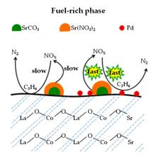
**Figure 8.** Possible NO<sub>x</sub> reduction routes on 1.4 wt % Pd/La<sub>0.7</sub>Sr<sub>0.3</sub>CoO<sub>3</sub> perovskite. Reprinted from [92]. Copyright (2018) American Chemical Society.
