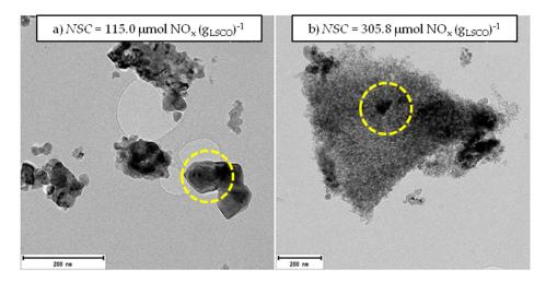
**Figure 4.** TEM images and NO<sub>x</sub> storage capacities (*NSC*) at 400 °C normalized per gram of perovskite of: (a) La<sub>0.7</sub>Sr<sub>0.3</sub>CoO<sub>3</sub> and (b) 30 wt % La<sub>0.7</sub>Sr<sub>0.3</sub>CoO<sub>3</sub>/Al<sub>2</sub>O<sub>3</sub> samples. Adapted from ref. [87]. Copyright (2018) Elsevier.
