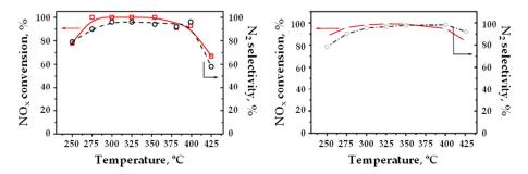
**Figure 7.** NO<sub>x</sub> conversion and N<sub>2</sub> selectivity of the La<sub>0.7</sub>Sr<sub>0.3</sub>Co<sub>0.97</sub>Pd<sub>0.03</sub>O<sub>3</sub> (left) and 1 wt % Pt–15 wt % Ba/Al<sub>2</sub>O<sub>3</sub> samples in the lean/rich cycles as a function of the operating temperatures with a space velocity of 32,000 h<sup>-1</sup>. Adapted from [67]. Copyright (2013) American Chemical Society.
