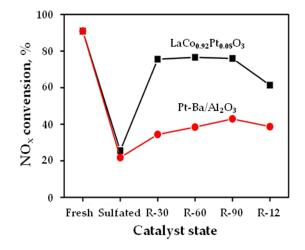
**Figure 10.** NO<sub>x</sub> conversion of LaCo<sub>0.92</sub>Pt<sub>0.08</sub>O<sub>3</sub> and 1 wt % Pt–16 wt % Ba/Al<sub>2</sub>O<sub>3</sub> at 350 °C for fresh, sulfated, and regenerated (R) catalysts. Reprinted from [70]. Copyright (2013) American Chemical Society.
