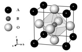
Figure 1. Ideal crystal structure of perovskite oxides with ABO3 composition.
