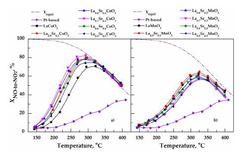
**Figure 2.** NO-to-NO<sub>2</sub> oxidation capacity of (**a**)  $La_{1-x}Sr_xCoO_3$  and (**b**)  $La_{1-x}Sr_xMnO_3$  perovskites with x ranging from 0 to 0.5, together with a model Pt-based catalyst. Reprinted from [25]. Copyright (2017) Elsevier.
