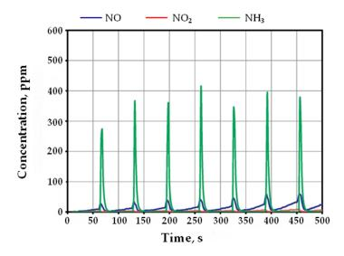
**Figure 6.** NO (blue), NO<sub>2</sub> (red) and NH<sub>3</sub> (green) concentration profiles at 350 °C under standard LNT test conditions with a GHSV = 25,000 h<sup>-1</sup>. Catalyst: Pd/Rh/LaMnO<sub>3</sub>/BaO/Al<sub>2</sub>O<sub>3</sub> (0 g/L Pt, 1.4 g/L Pd, 0.2 g/L Rh). Reprinted from [72]. Copyright (2012) Elsevier.
