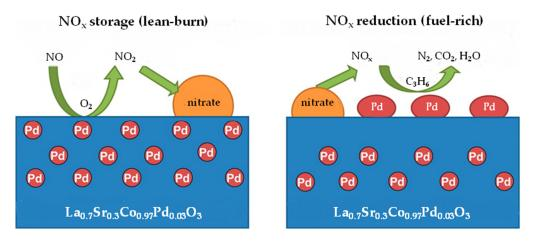
**Figure 9.** NO<sub>x</sub> storage and reduction routes and Pd mobility scheme on for  $La_{0.7}Sr_{0.3}Co_{0.97}Pd_{0.03}O_3$  perovskite during alternative lean-rich cycles. Reprinted from [67]. Copyright (2013) American Chemical Society.
