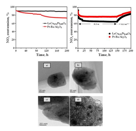
**Figure 11.** Thermal stability (left) and stability tests with 10 vol%  $H_2O$  (right) at 350 °C of  $LaCo_{0.92}Pt_{0.08}O_3$  and  $Pt-Ba/Al_2O_3$ . TEM images for (**a**)  $LaCo_{0.92}Pt_{0.08}O_3$ , (**c**)  $Pt-Ba/Al_2O_3$ , (**b**) aged  $LaCo_{0.92}Pt_{0.08}O_3$ , and (**d**) aged  $Pt-Ba/Al_2O_3$ , which were maintained at 850 °C for 40 h followed by  $NO_x$  conversion test at 350 °C for 200 h. Reprinted from [70]. Copyright (2013) American Chemical Society.
