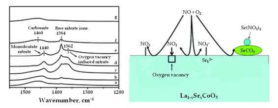
**Figure 3.** FT-IR spectra (left side figure) of  $La_{0.7}Sr_{0.3}CoO_3$ : fresh (**a**); after NO<sub>x</sub> storage at 200 °C (**b**); 250 °C (**c**); 300 °C (**d**); 350 °C (**e**); and 400 °C (**f**); the sample (**c**) reduced by 5% H<sub>2</sub> at 300 °C for 10 min (**g**). Possible NO<sub>x</sub> storage routes (right side figure) on  $La_{1-x}Sr_xCoO_3$  perovskites. Adapted from [66]. Copyright (2011) The Royal Society of Chemistry.
