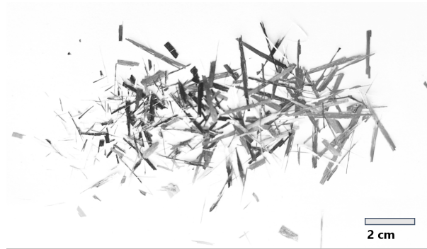
Figure 3.2: Photograph of the \text{Sm}_{0.5}\text{Ce}_{0.5}\text{Fe}_9\text{Co}_2\text{Ti} as-spun ribbons. The thickness was 30 \mu\text{m} approximately.
