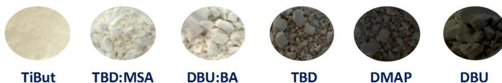
**Figure 3.5.** Pictures of PET synthesized with different catalysts.
