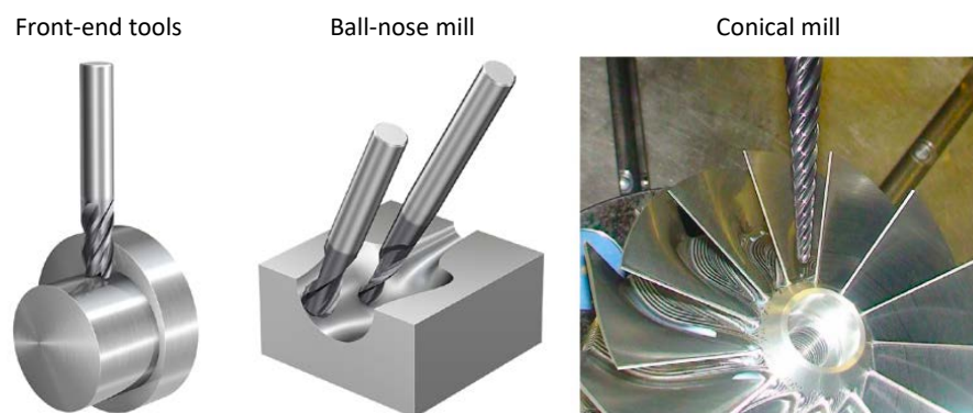
Figure 9. Sandvik® [45] and Emuge-Franken® [47] milling cutting tool forms for IBRs manufacturing.
