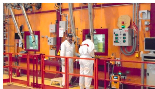
Example of hot cells front area : hot cells for research and development activities on fuel.
