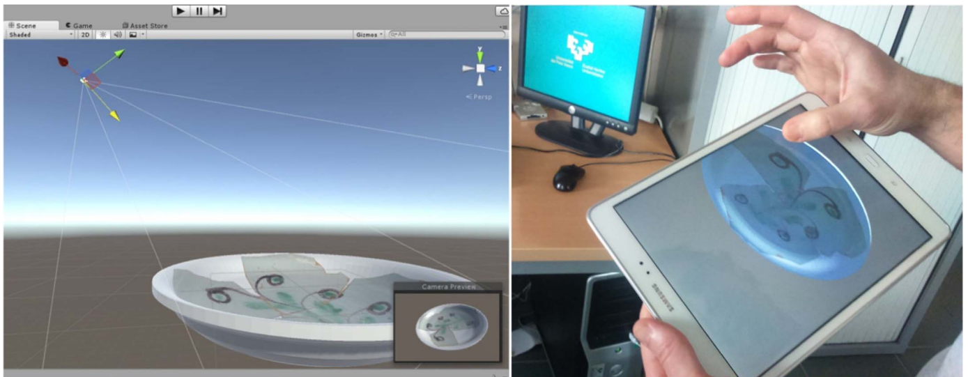
Fig. 8. The image on the left shows one of the models imported in an environment for graphic design ( Unity 3D ®) from which the application shown in the image of the right was created. This application permits haptic interaction with the virtual object through a tablet.
