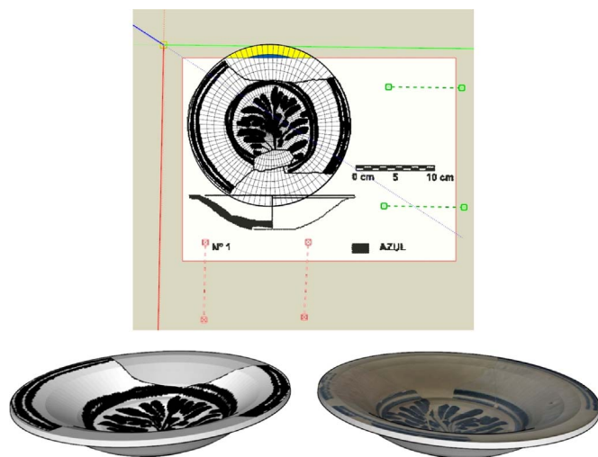
Fig. 5. Handmade drawing (on top) from which geometry and texture can be obtained (bottom left model). The same geometry can be also wrapped with textures from other sources such as photographs (bottom right model).
