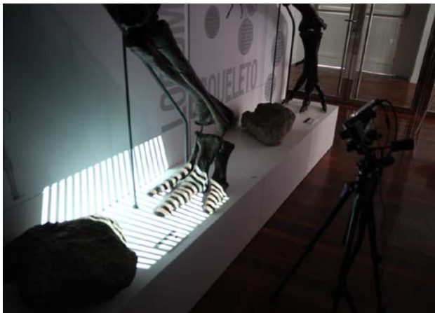
Figure 5.- Fringe projection during the 3D data acquisition with the "Scan in a Box" device.
