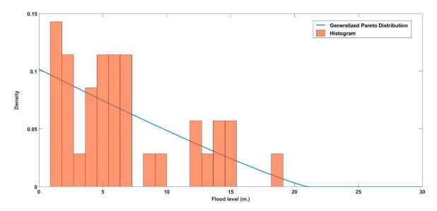
Figure 2. Flood level with generalized Pareto distribution.
