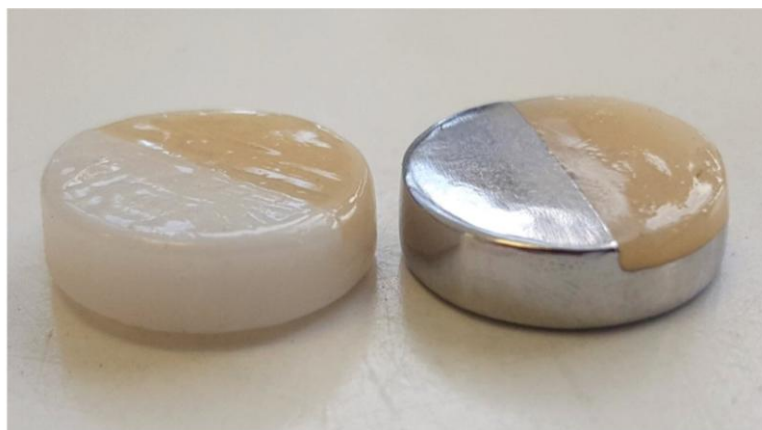
Figure 1. Discs half-covered with Ls2 ceramic prepared to observe the features of the junction area by SEM.
