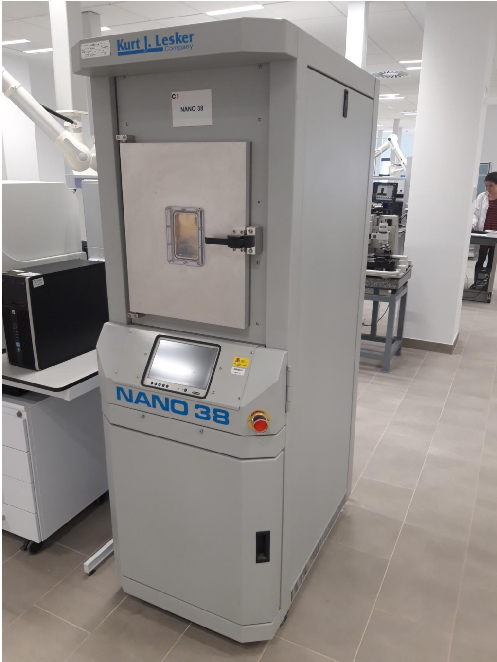
Figure 2.3. Photograph of a thermal evaporator used in this thesis for the evaporation of the top contacts of PSCs.
