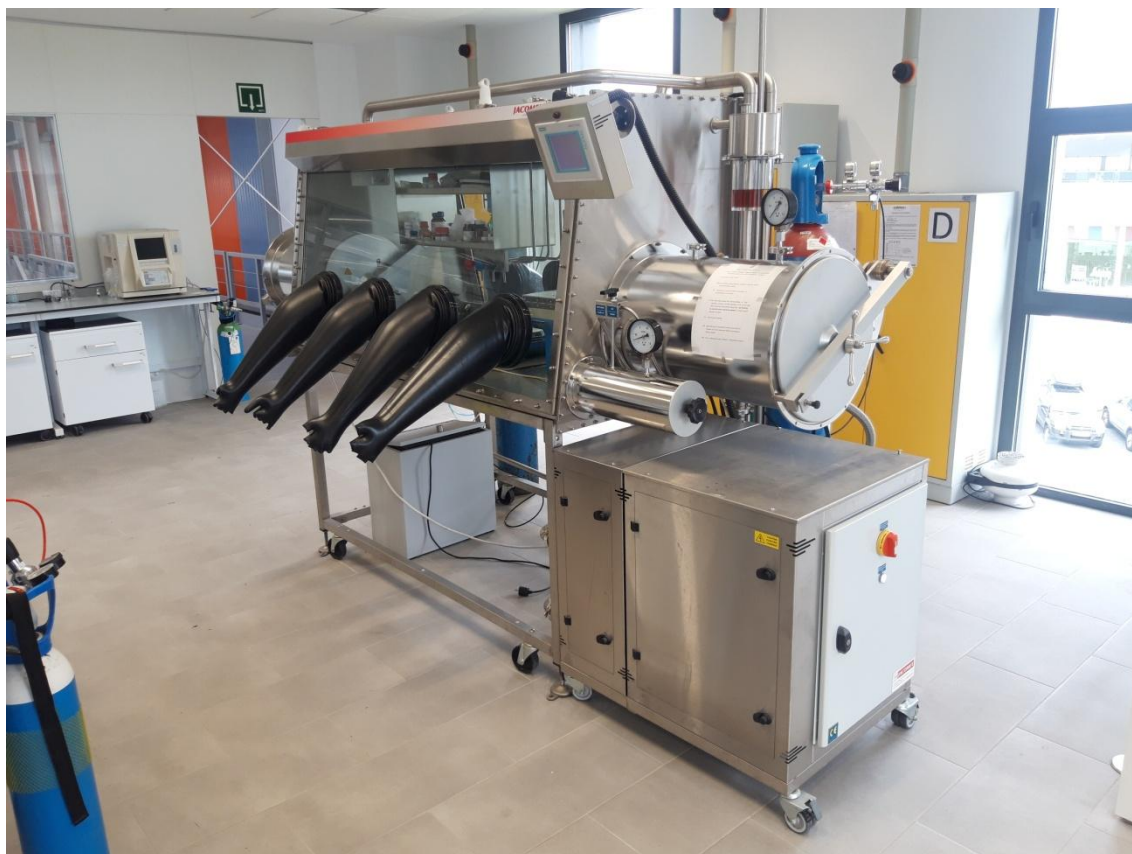
Figure 2.1. Photograph of a glove box used in this thesis for the processing of perovskite materials.
