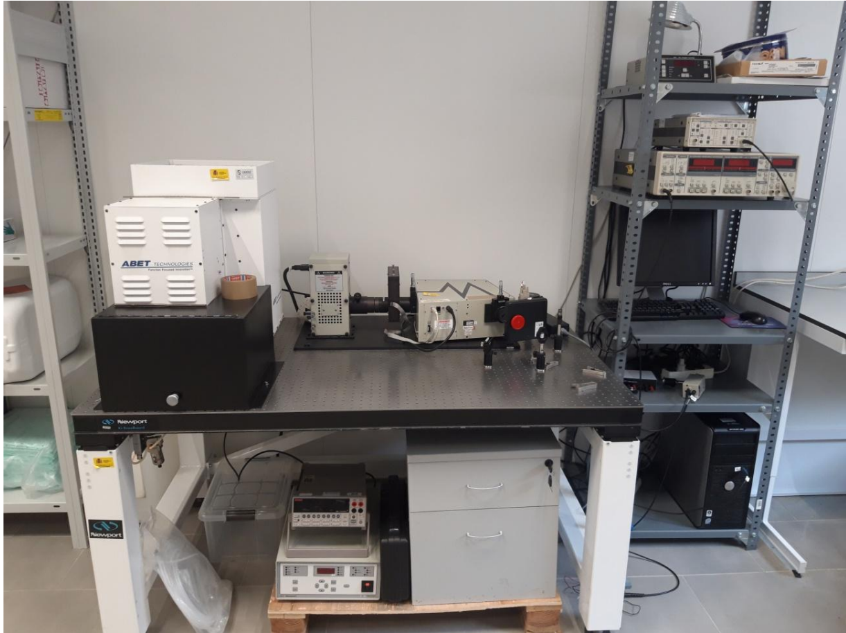
Figure 2.4. Photograph of a sun simulator and EQE setup used in this thesis for the PV characterization of PSCs.
