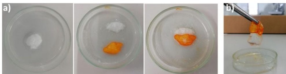
Figure 3. Self-healing process of chitosan and hyaluronic-acid-based polycomplex, (a) cut and repairing process of the system, and (b) repaired hydrogel. Reprinted with permission from N. Barroso et al. Self-healable hyaluronic acid/chitosan polyelectrolyte complex hydrogels and multilayers [51]. Copyright © (2020), with permission from Elsevier.
