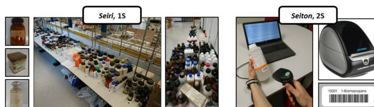
Figure 4. Sort (1S) and set in order (2S) steps of 5S methodology application.
