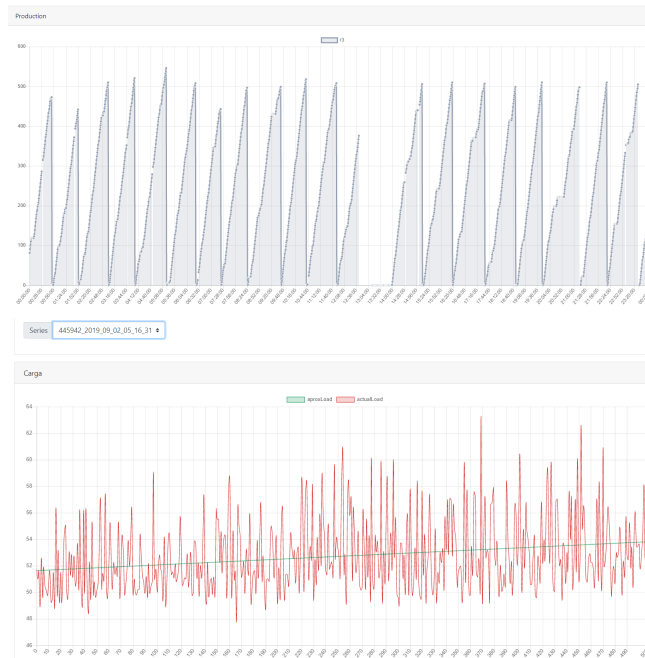
Figure 5: Application integrated at the machine showing the Remaining Useful Life (RUL) for the actual working tool.
