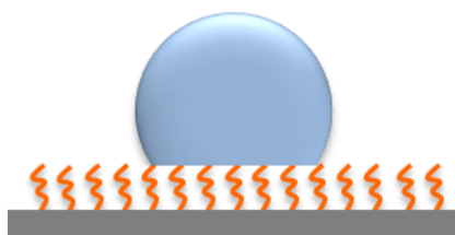
Figure 1.6. Schematics of flat surfaces grafted with liquid-like molecules (SOCAL surfaces).
