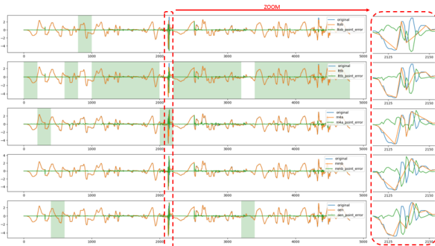
FIGURE 7: y_o (in blue), y_r (in orange), y_r - y_o (in green) time series from a synthetically generated time series. The optimal method selected by PRD in each window is highlighted. At right, a detailed view of a representative time segment is added.
