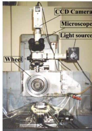
Figure 23: Automatic image processing device implemented on surface grinding machine [88]
