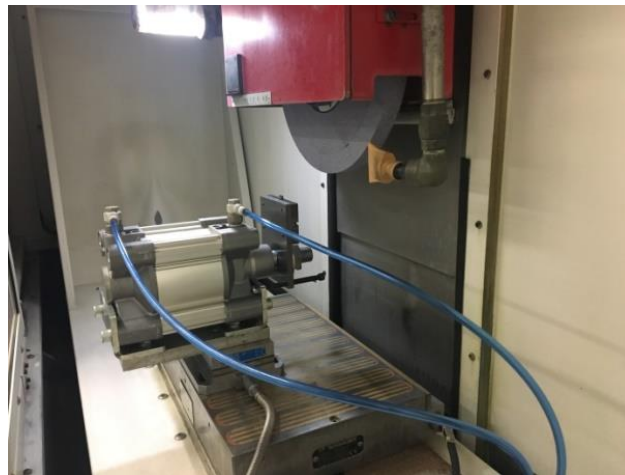
Figure 54: Set up of tribometer mounted on a surface grinding machine.
