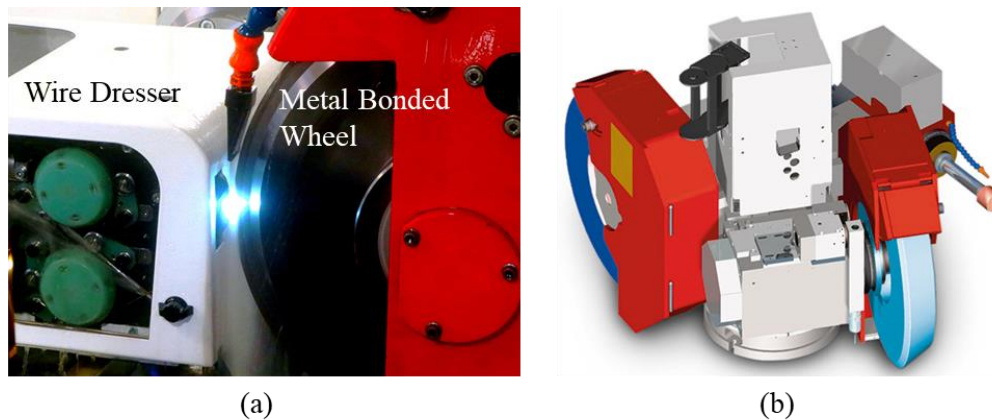
Figure 3: (a) Wire Dress system developed by Studer company, integrated on grinding machines, (b) tool exchange of Studer S33 grinding machine [6]
