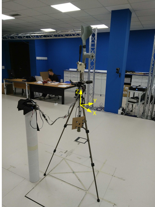
Figure 3.18: Experimental setup for the calibration of the inclinometer. A tripod with a clamp and an integrated protractor is used to keep the crutch static with a constant tilt angle while the MCS records the positions of the markers.
