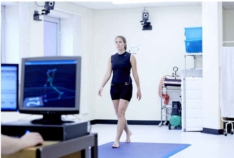
Figure 2.3: Vicon MCS, showing the 3D kinematics of the two legs.
