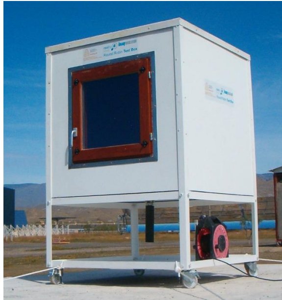
Figure 7. The small scale “building” named Round Robin Box.
