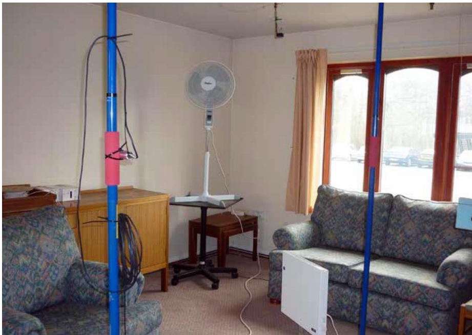
Figure 2. Example of a typical co-heating configuration. [27]
