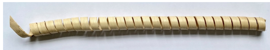
Figure 15. 80 cm strip immersed for 24 h and wound onto a 1 cm radius cylinder until dry.
