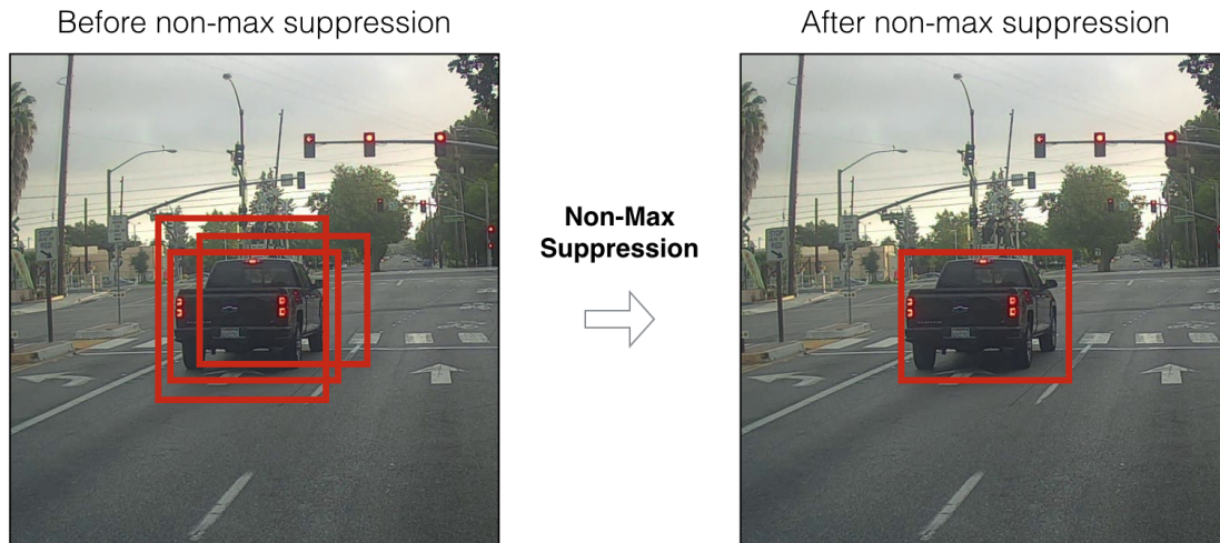
Figure 2.6: Non-maximum suppression example removing the surplus predictions (left) and leaving the best one for the given object (right). Source: https://towardsdatascience.com/non-maximum-suppression-nms-93ce178e177c
