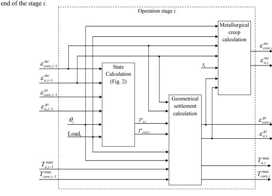
Fig. 9. Creep calculation in the operation stage i
