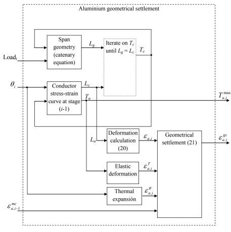
Fig. 10. Aluminium geometrical settlement calculation in the operation stage i
