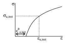
Fig. 5. Modified (1 h metallurgical creep removed) aluminium stress-strain curve
