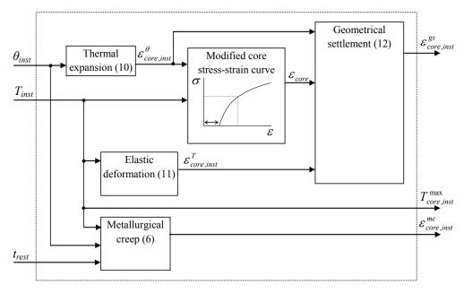
Fig. 6. Creep developed in the core of a gap-type conductor during the installation
