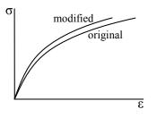
Fig. 4. Modified (1 h metallurgical creep removed) stress-strain curve
