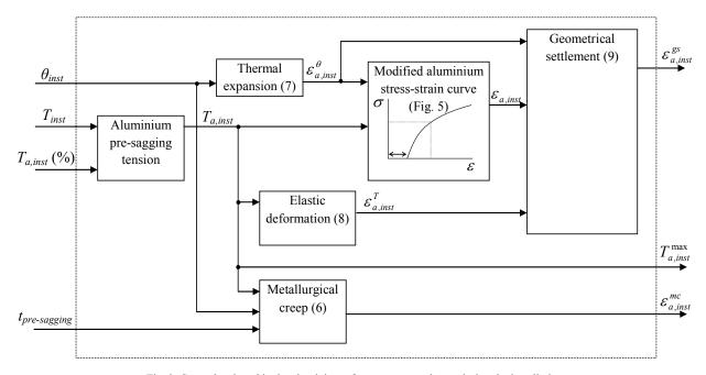
Fig. 3. Creep developed in the aluminium of a gap-type conductor during the installation
