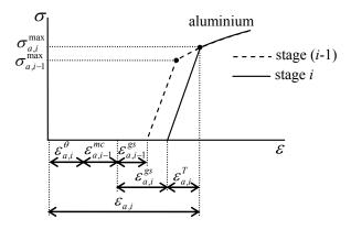
Fig. 11. Stress-strain curve of the aluminium at the end of the stages (i-1) and i
