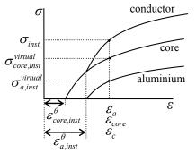
Fig. 8. Modified conductor stress-strain curve
