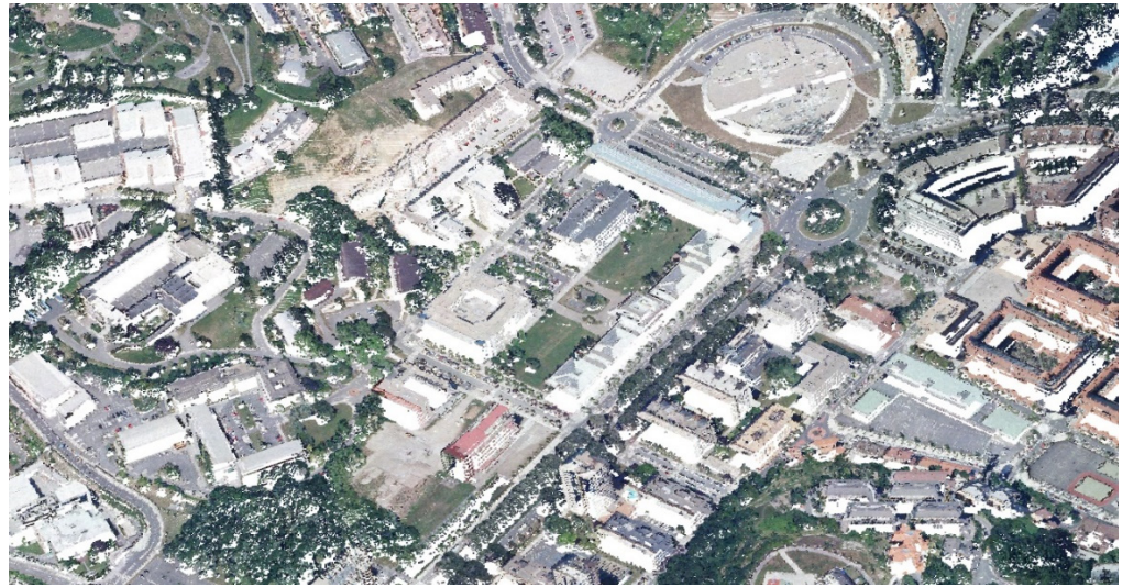
Figure 5. 2012 flight LiDAR point cloud of the UPV/EHU university campus in DSS. Cloud density: 1 point/m 2 .
