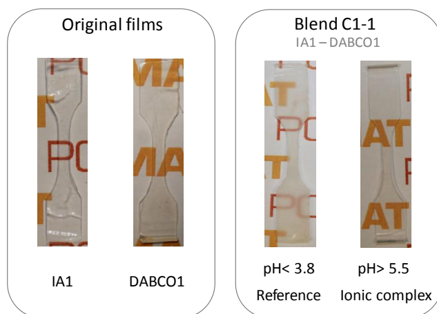
Figure 4.5. Appearance of the individual polymers (IA1 and DABCO1) and the blend C1-1 films at different pH's (reference and ionic complex).
