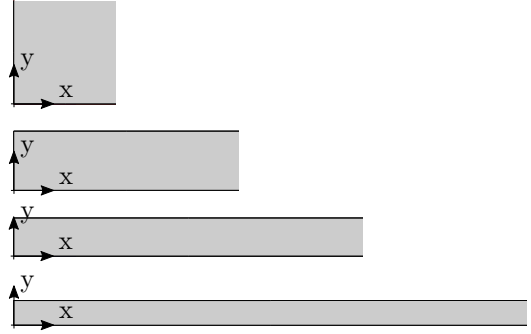
(b) Deformation history of the single element tensile test in a LD framework.
