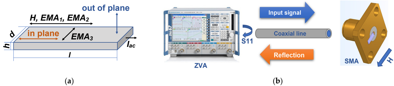
Figure 1. (a) Schematic description of amorphous ribbon sample with dimensions l \times d \times h : H is the external magnetic field applied during magnetic and GMI measurements, however for FMR measurements in the resonance cavity both in-plane and out-of-plane orientations of the external magnetic field were used; EMA_1 corresponds to the easy magnetization axis of the sample in initial state; EMA_2 corresponds to the easy magnetization axis of the sample after relaxation annealing; and EMA_3 corresponds to the easy magnetization axis of the sample after TMO. (b) The scheme of the broadband microwave measurements using ZVA VNA for the coaxial position of a sample; H is an external magnetic field.
