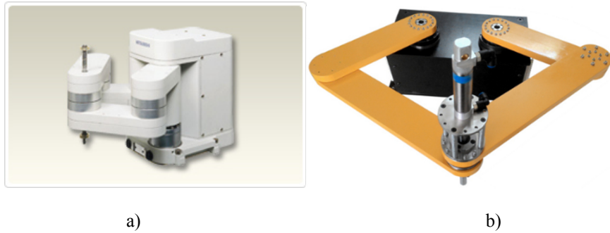
Figure 42. SCARA-type parallel manipulators: a) Mitsubishi Electric High precision SCARA parallel robot [91]; Gridbots RAPI-MOV [92].
