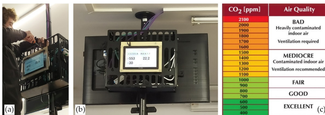
Figure 9. Pictures (a,b) show the set-up of the displays that provided real-time feedback to the students in rooms A 1.1 and A 2.1, while (c) reproduces the legend installed in both classrooms and the administration office. Source: authors.
