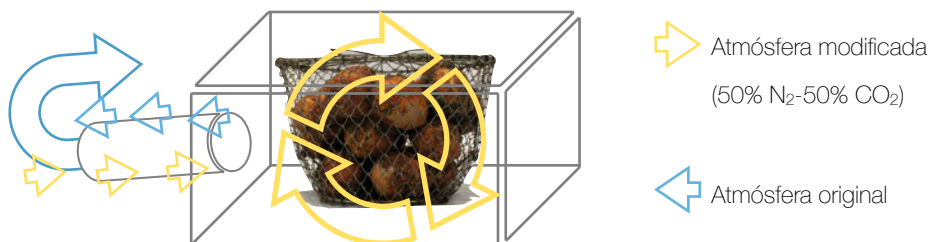
[F. 96] Diagram of the installation of the new atmosphere in the container that stores the work.
