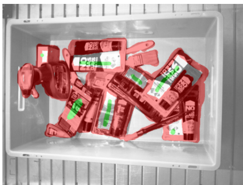
(a) Suction annotation in RGB-D data. Green and red pixels belong to good and bad grasping areas respectively. Remaining pixels are considered as neutral. (b) Same scene converted to semantically annotated point cloud. Green, blue and pink points belong to good, bad, and neutral grasping areas respectively.
