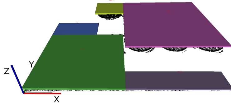
Fig. 5.9.: Projections of the cubic solutions that represent the empty space inside the bin.
