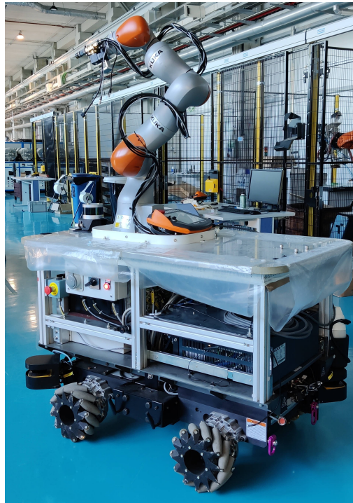
Fig. 1: The robot, developed by Tekniker, combines a commercial Segway omnidirectional mobile platform and a KUKA iiwa arm.
