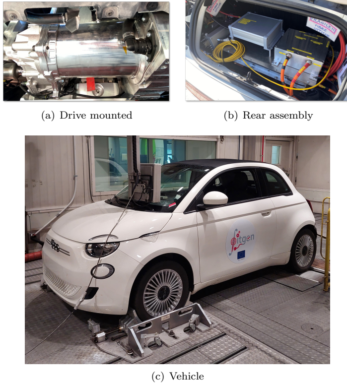
Fig. 4.35: Electric vehicle used to carry out the verification of the proposed control approach under standardized driving cycles.
