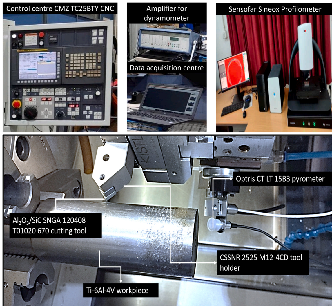
Fig. 2. Experimental setup for dry turning of Ti-6Al-4 V titanium alloy.
