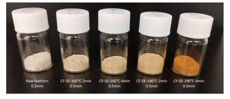
Figure 1. Digital images of the CF treated at different SE conditions.
