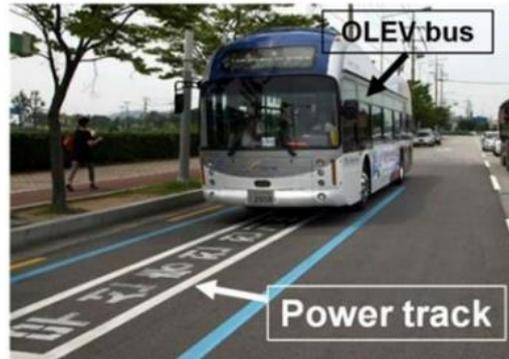
**Fig. 4.** On-line Electrical Vehicle (OLEV). [3]
