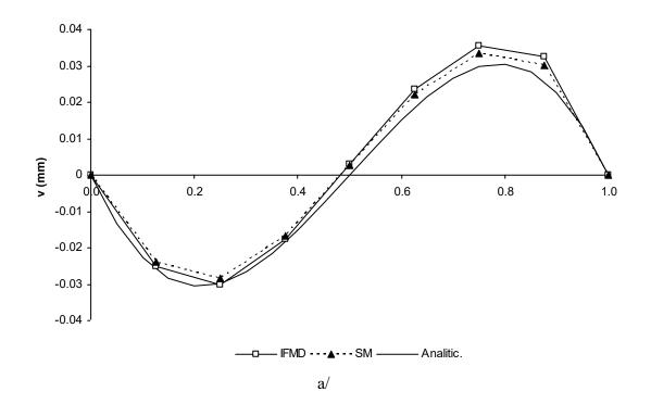
Figure 7. Displacements in the off-axis tensile specimen: a/Horizontal displacements, u; b/Vertical displacements, v.
