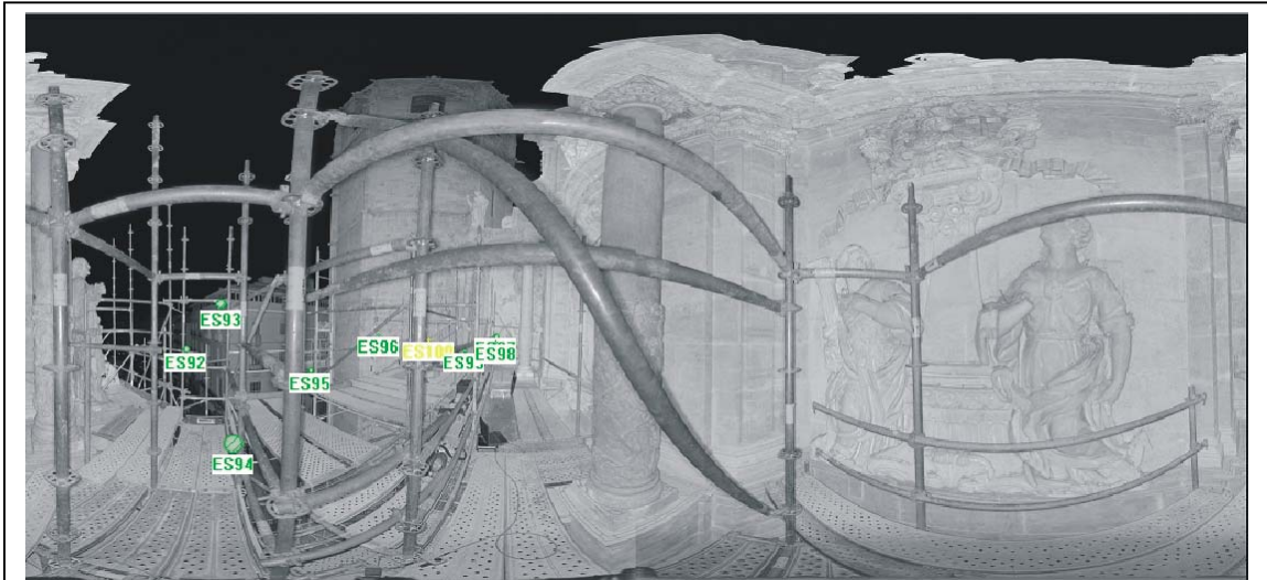
Fig. 3.- Scan orientation by identifying the visible benchmarks.
