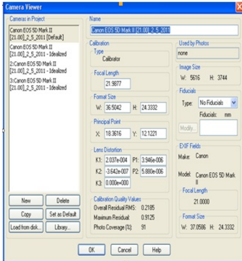
Image_18: Calibration results of Photomodeler Scanner 6
