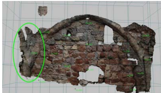
Image_39: The corner as it appears at the model of the eastern wall
